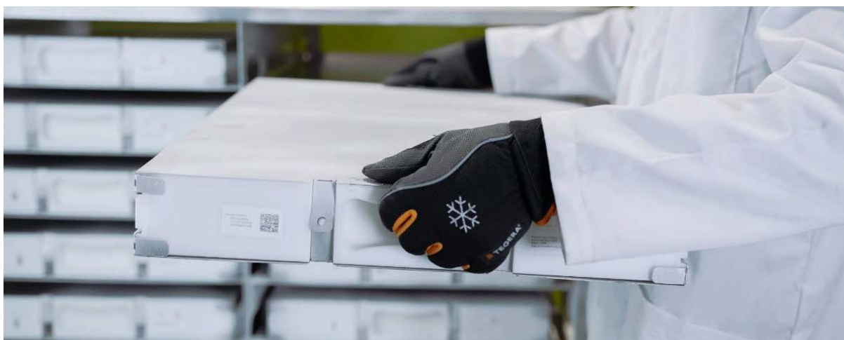
Figure 2: Frozen drug substance handling in single-use bags can be manual or supported by full-batch processes
