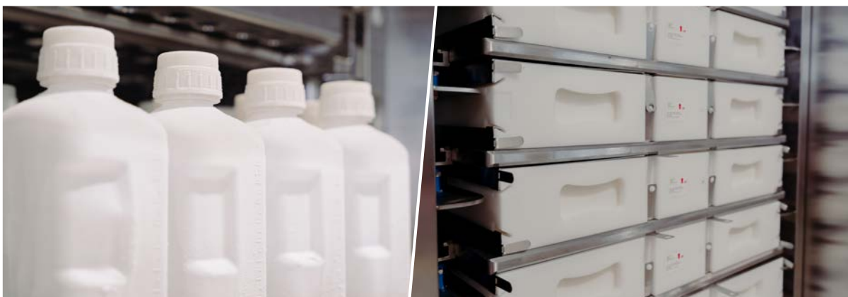
Figure 3: Single-use bottles are typically frozen in blast freezers (L), while single-use bags are often frozen in plate freezers (r.)
