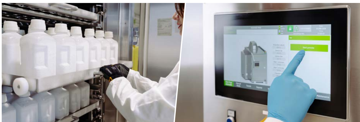
Figure 5: Modular interior with shelves or full trolleys with RoSS.BLST controlled freezing of bottles and bags.
