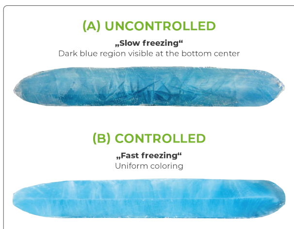
Figure 2: Image showing the clear homogenous freezing in RoSS® shells, whereas uncontrolled slow freezing negatively affects critical quality attributes due to the occurrence of cryoconcentration
