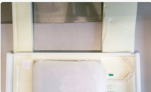
Figure 4: RoSS® shell 1049 at 4.5 L filling volume after freezing, showing foam impressions generated during freezing
