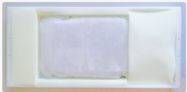
Figure 5: RoSS® shell 1013 at 4.2 L filling volume after freezing, showing positioning of the bag assembly within the shell
