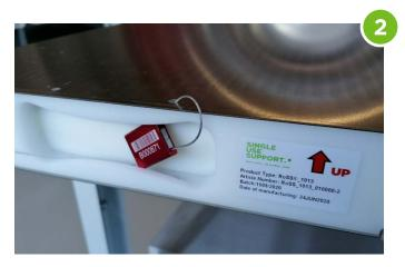
**Tied through lid:** Either cable ties or galvanized steel wires are used to secure both lids with front panel.
