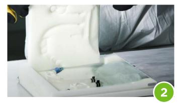
interior is lined with specialized foam inlays that provide additional stabilization. The 3D foam offers a protective enclosure for the single-use bag and its attachments. But it also absorbs the bag's/liquid's expanding energy caused by the density drop during freezing. At sub-zero temperatures, when the bag is already frozen, the foam hardens. The bag is fully immobilized in the hardened foam setup, making it safe to handle during storage and shipping.
