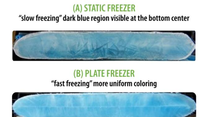
Figure 1: Comparison slow (A) vs. fast freezing (B): Increased cryoconcentration at slow freezing
