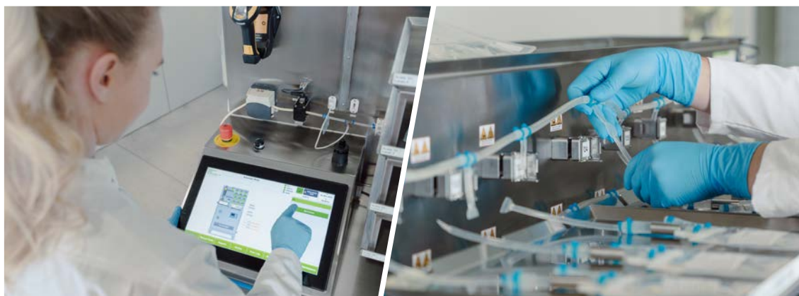
Figure 4: RoSS.FILL precisely fills high-value biologics into single-use bags and bottles with aseptic sealing valves.
