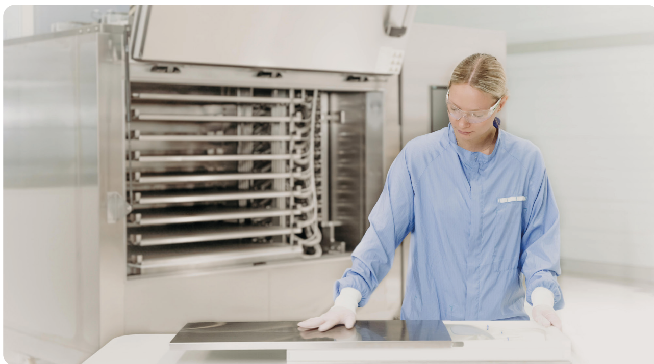
The RoSS® shell protecting 2D single-use bags during filling and freezing.
