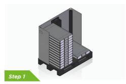
Place the RoSS® shells in the correct position in two predefined piles. *Note:* keep one side wall in place to guarantee a proper positioning.
