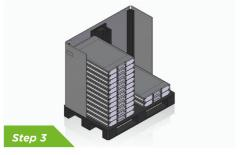
Continue adding RoSS® shells and anti-sliding pads. *Note:* Make sure that the shells are stacked ordely on top of each other.
