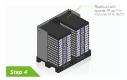
If the RoSS.RACK is not filled up with 26 RoSS shells, fill the remaining volume with replacement spacer.
