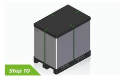
Adjust and tighten strapping belts to prepare RoSS.RACK for final shipment.
