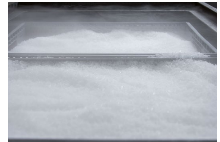
RoSS.SHIP (single-use) test run Worst-case test (empty) 100kg dry ice loading
