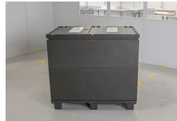
RoSS.SHIP (single-use) test run Worst-case test (empty) 100kg dry ice loading
