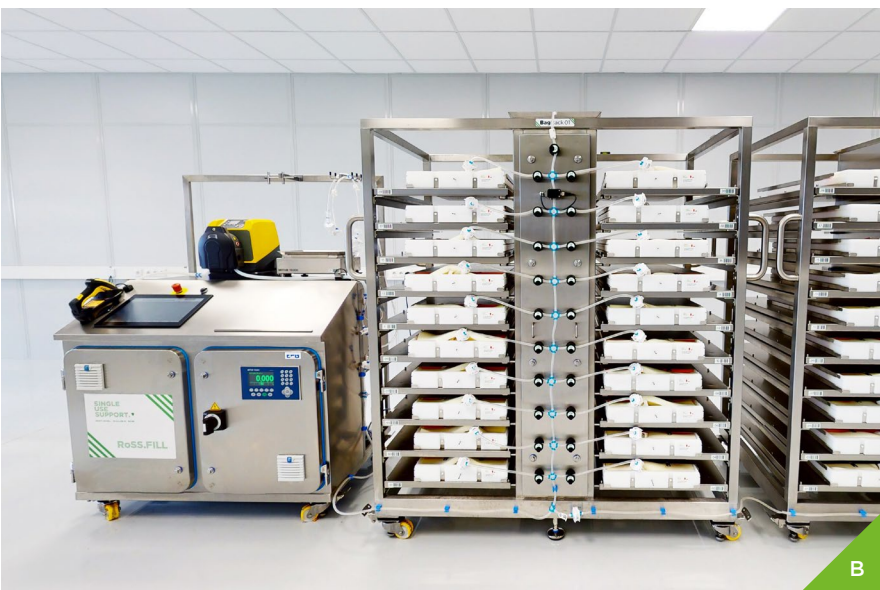
Image 2: Modularity enables hybrid filling with (A) RoSS.FILL Bottle and (B) RoSS.FILL Bag
