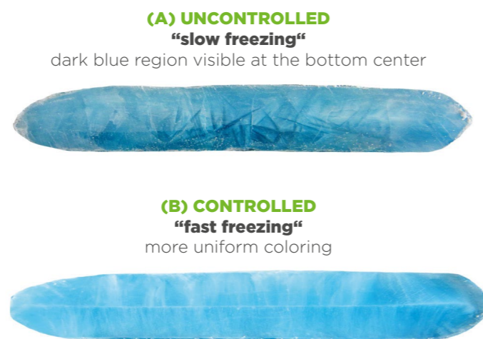
Figure 1: Comparison slow (A) vs. fast freezing (B): Increased cryoconcentration at slow freezing
