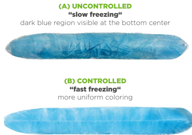
Figure 2: Comparison slow (A) vs. fast freezing (B): Increased cryoconcentration at slow freezing
