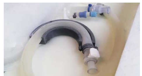
Figure 14: Tubing guide inside RoSS® shell
