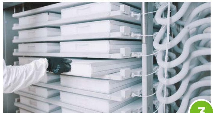
Figure 4: Frozen RoSS® shells in Single Use Support's plate freezer RoSS.pFTU Large Scale
